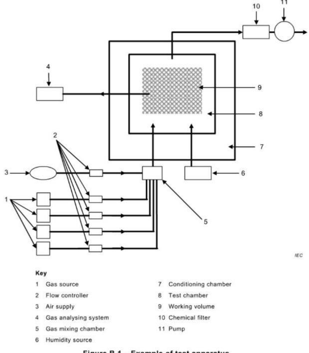
Figure B.1 - Example of test apparatus
